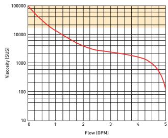
Note 1: Guardian not recommended for fluid viscosities greater than 16,000 SUS (11,000 SUS;24VDC)
