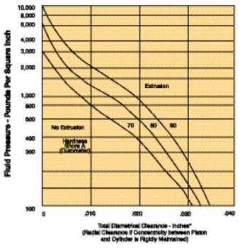
Extrusion-Pressure/ Hardness/Clearance-gap Relationships
