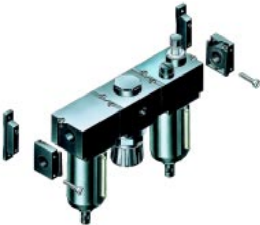
Wall brackets mounted at the ends of an assembly
